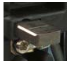
Visual inspection of carbon brushes is rather simple due to the markings as applied.
